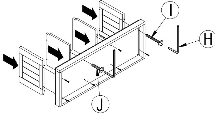
4. Insert the Back panel (D) as shown.
