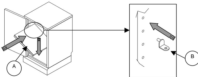
3. Gently tilt the shelf by lowering the other end of the shelf until it seats onto the shelf pegs (B). Hold the other end in upright position and insert two shelf pegs (B) into the pre-drilled holes until fully inserted. (Fig 2)
