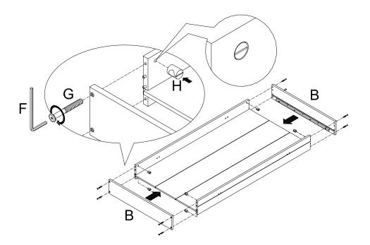
4. Turn trundle upside down. Secure bottom boards with the Long/Short side panel using the Small Phillips head screw 8x25mm (J).
