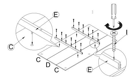
2. Turn assembled base right side up, Insert the wooden dowels on the ends of the Cross bars (E) into the pre- drilled holes on the Long side panel (A) as shown. Press firmly to ensure the left and right Bottom boards (C) sit in the slots of the Long side panel (A).
