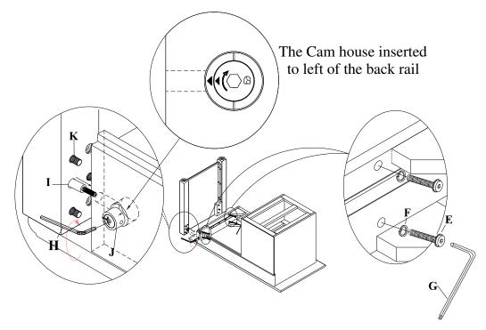
4. Put a Cam House (J) into notch at the other end of back rail, ensure arrows on the cam house pointing at pre-drilled hole in the notch for cam house. Align wooden dowels and Cam Stud on Right End Panel (C) with pre-drilled holes in end panel of the desk top drawer compartment, tighten cam house with Allen Key (H) as shown below.
