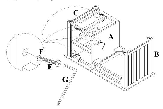
6. Attach Turning Legs (D) to Left and Right End Panels (B&C) as shown below.
