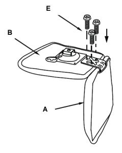
NOTE: when performing assembly of the back to the seat, please push the bracket on the back in order to have the holes on the bracket align with the holes on the seat. 4. Insert assembled seat onto top of Gas Lift Post (D) by pressing firmly.
