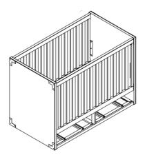
15. Attach (Q&R) to (H) using (N). Make sure the brackets point outwards as shown below.
