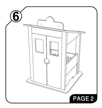
You may turn slightly any of the four vertical posts (B, C, D, and E) to help align the doors, as necessary.
