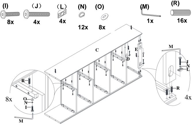
Attach Dowel 8 x 30mm (R) on top of Side panel, Front Frame, and Back Frame. Then assemble Top panel (A), using JCBC Bolts M6 x 32mm (I), Lock Washer (N), and Flat washer (O). Tighten the Bolts with Allen Key (M). At the same time, insert the Round Head Screw 8 x 38mm (Q) to the Front Frame (D) and Back Frame (E) hole (at the center). Tighten the screws using a Phillips screw driver (not included).
