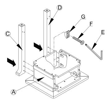
3. Attach the Bottom panel (B) to the Leg (C) and (D) using 2pcs Allen bolt 1/4"x38x11.5mm (F) and 2pcs Half moon washer 1/4"x24x8mm (G), tighten with Allen key (E).
