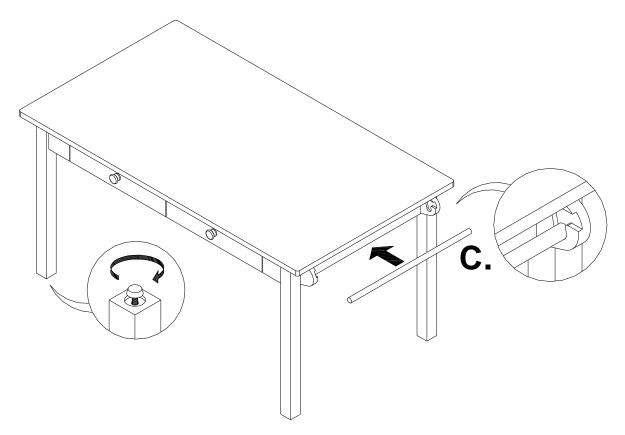
3. Adjust levelers on bottom of legs to keep table level when needed.
