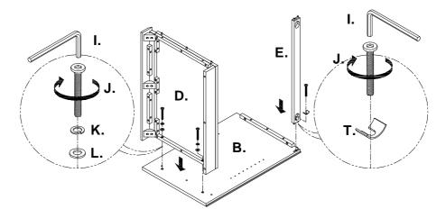
Repeat the above steps to secure the Right Side Panel (C) to the Bottom Panel and the Rear Top Rail.
