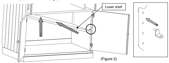
3. Gently lower the shelf and rest it onto the shelf pins. Fasten the screws using a Phillips head screwdriver. (Fig 3)
