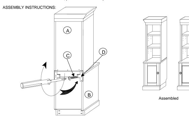
1. Carefully raise the hutch (A) with another person and set onto the top of the desk (B). Attach the connection plates (D) by aligning the plates with the pre-drilled pilot holes. Use CBS screws (C) to fasten the connections.
