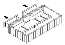
7. If only one drawer is needed, replace that open drawer front using the drawer Fill-in panel (G), make sure the bead board aligns properly for both the Front panel (A) and Drawer Fill-in panel (G), then fix 2pcs Mending plate 70x40mm (L) through the pre-drilled holes by using 8pcs Small Phillips head screw 8x17mm (K) and Phillips head screwdriver (not included).
