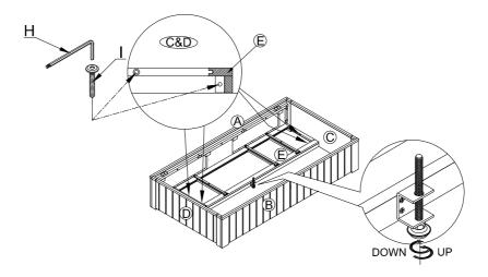
6. Put the drawer boxes back to the Bottom frame (E) by aligning the wooden runners making sure the drawer fits properly.
