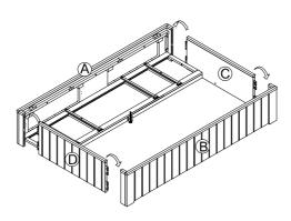
5. Fix the Bottom frame (E) to Left Side panel (C) and Right Side panel (D) using 4pcs Allen bolt 1/4"x32x15mm (I), tighten with Allen key (H). Then tighten the leveler as shown.
