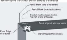
Step 3: To prevent any wood from splitting when screws are secure therein, we recommend that pilot holes be drilled at the marked locations for the brackets. Use a power drill and a 1/8 inch drill bit to drill a hole at each mark
