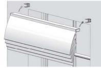
Step 7: Once the headrail is properly centered within the brackets, use a screwdriver and a provided short screw to secure the mounted headrail to each end bracket (securement to the third central bracket, if there is one, is not necessary).
