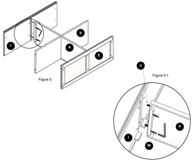
6. Attach the Right Side Panel (D) and the Left Side Panel (C) to the already assembled body with eight (8) Wood Dowels (O), two (2) on both ends of the Bottom Panel (E), and two (2) on both ends of the Divider (B). Secure Divider (B) to the Left and Right Side Panels (C & D) with four (4) Short Bolt & Washer Sets (M) using Allen Key. Then, connect the Bottom Panel (E) to the Side Panels (C & D) with four (4) Long Screws (P) using Philips Screwdriver (not included). (See figures 6, 6-1 & 6-2).
