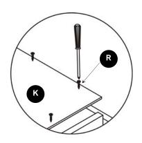
10. Attach the four (4) Doors (L) to the Left and Ride Side Panels (C & D) with six (6) Short Screws (R) on each door using the Phillips Screwdriver (not included). Match-up the color of the door to the corresponding color of the cubby. (See figures 10 & 10-1).
