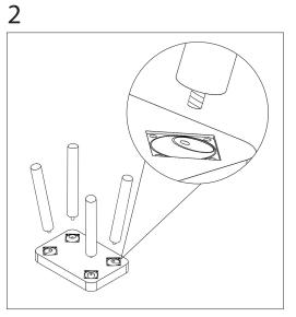
Screw in stool legs (B) to round seat top (A) as seen in image. Adjust until tight.
