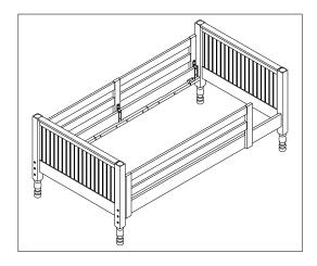
4. Fasten guardrails (D) and (E) to side rails (C) of upper bunk using Screws (R). The long guardrail goes on the back side rail of the upper bed. Make sure there is no gap in between the other end of the short guardrail (D) and the bed end structure (A) before you start screwing the brackets to the front side rail. Turn brackets on bottom of guardrails and secure to underside of bed rails as shown. Use Phillips head screwdriver for tighten screws.
