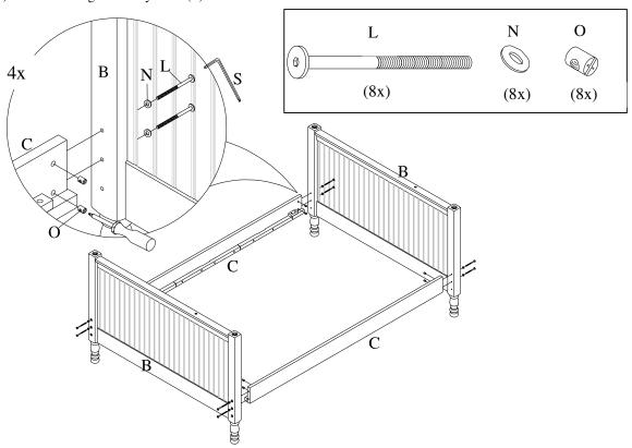
2. Assemble upper bed using short end (A) and two side rails (C) using JCBC 6 x 110mm Allen bolts (L), Flat washer (N) and Barrel Nut (M) as shown using Allen key (S).
