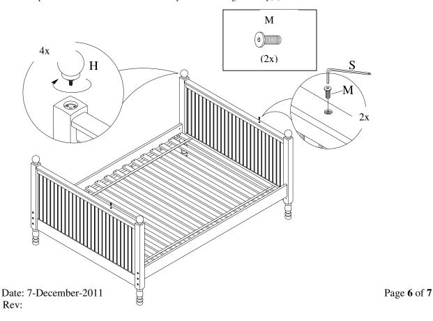
10. If used with trundle bed (sold separately), make sure you assemble the bed with the side rails in the upper set of holes as shown.
