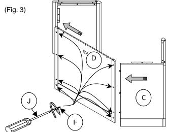
3. Align the pre-drilled holes of the Front Side Panel Left & Right (B) & Back Side Panel Left & Right (C) & Back Panel (D) with those on the Top Panel (A). Insert a JCBC Screw (E), Spring Washer (G), and Flat Washer (F) through the pre-drilled holes of the Front Side Panel Left & Right (B) & Back Side Panel Left & Right (C) and into the pre-drilled holes of the Top Panel (A). Tighten using the Allen Key (K).(Fig. 4) Repeat the same step (Fig. 5)
