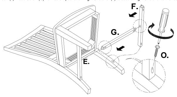
4. Connect Right Front Leg (D) to corner of Chair Seat and align opening on the leg to Right Stretcher (F). Secure the leg to the Chair Seat with a Flat Washer (M), a Spring Washer (L) and a Nut (N) using Wrench (I). Insert (1) Wood Screw (O) from screw pocket on Right Stretcher (F) to secure Right Stretcher (F) to Right Front Leg (D).
