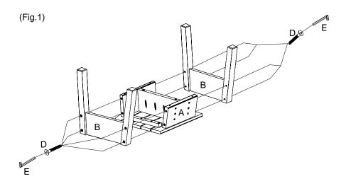
2. Upright the chair, then secure the backrest (C) to seat (A) with 4 bolts (D). Make sure all bolts are in the correct position, then tighten all bolts using Allen Key (E).
