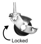
To lock the casters, rotate clockwise To unlock casters, rotate counter clockwise
