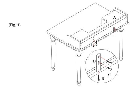
2 Adjust the Adjustable Levelers on the bottom of the Legs by loosening or tightening them so the Table sits evenly on floor.
