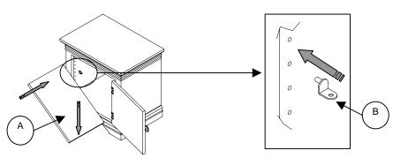
3. Gently tilt the shelf by lowering the raised end of the shelf until it rests on the shelf pegs. Hold the free end of the shelf in an upright position and insert the remaining (2) Shelf pegs (B) into the pre-drilled holes until fully inserted. (Fig 2)
