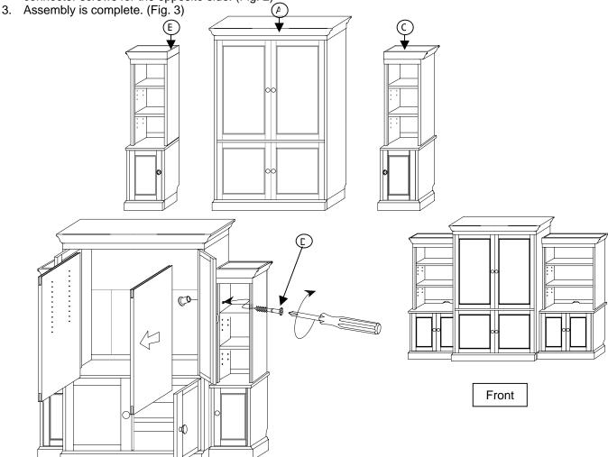
Note: The wall system should not be moved unless the connector screws are removed.
