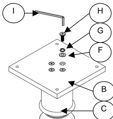
4. Attach the Tabletop (A) to the Connector Plate (B) and fasten the Flat washer (F), Spring washer (G) and JCBC Bolt (H) at each connection point with the Allen key. (Fig. 4)
